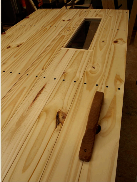
Above: Pine-panel front door under construction (the cherry handle is hand-carved). A view of the mountains from breakfast-area window. Facing page: My daughter Sarah visits the construction site during Thanksgiving 2008. Kevin textures a wall. Siding almost done.
